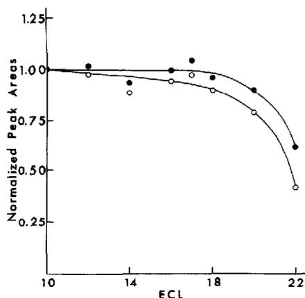
Fig. 2. Relationship between peak area and equivalent chain length (ECL) of cholesteryl esters chromatographed on: ●, DB-1 fused silica column, GC conditions in Fig. 1; ○, SP2330 column, GC conditions in Fig. 3.
